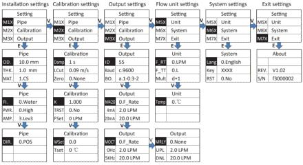
Menu setting operation: press  $\, \lor \,$  to select setting menu, press E to enter menu setting, press  $\, \lor \,$  to enter number or option, press E to save and exit setting
