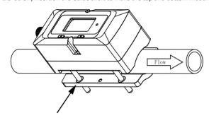
2.4 Lock screws to fix the host, do not over lock, to avoid damage to the Coupling pad.
