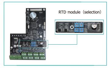
The LRF-3000S can be used in conjunction with the RTD module and the PT1000 temperature sensor to become an energy meter for measuring the heat and cold consumption of heating pipelines and air-conditioning refrigeration pipelines;
